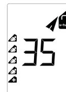
**SCROLLING MODE:** when scrolling mode is activated (see paragraph 1.5/ SETTING UP YOUR DEVICE), you have the option to select the burial you want to target. Use the "+" and "-" buttons to select the burial you want to target (the pictogram corresponding to this burial will blink). **Please note that this mode is reserved for expert users with advanced avalanche rescue skills.**
