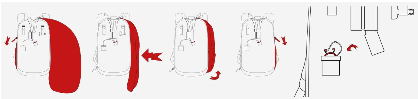
6/Carry on folding the rest of the airbags as shown in the illustrations, then close the 2 slide fasteners to the bottom of the bag.
