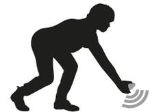
2. Move your device in a cross pattern to locate the point where the distance reading is the lowest.
