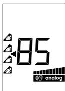
The left and right arrows blink alternately to help the user choose the correct calibration. If you press the marking button, you return to automatic sensitivity calibration management. At sensitivity level 10 (the highest), the screen switches itself off to limit the level of interference and provide maximum detection performance.
