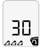
In a complex situation where there are multiple burials or in an environment where there is a lot of interference, the device might reach analysis overload. In this case, distance yourself from that specific area and then return by following another direction.
